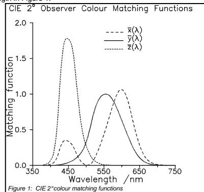
CIE luminosity function  $V(\lambda)$ , so that the value at 555 nm is 1.00,  $\overline{y}(555)=1.000$ .
