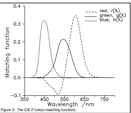
The appearance of the de-saturated monochromatic light could then be matched by a combination of the other two primaries. When this occurs the amount of the primary added to the monochromatic light appears as a negative number in the colour specification.
