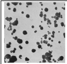
Figure 13: Particles of a Furnace black. Mag. 16,000
