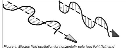
Figure 4: Electric field oscillation for horizontally polarised light (left) and vertically polarised light (right)
