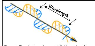
Figure 1: The electric and magnetic field variation of an electromagnetic wave travelling through space
