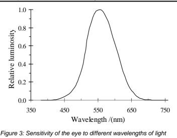
The luminous efficiency of a lamp describes the fraction of the electrical energy that is converted to useful visual energy and has the unit of lumens/Watt. The luminous efficiency value depends on the *spectral power distribution*, the relative energy emitted by the lamp at each wavelength in the visible spectrum. The most efficient of the commonly available types of lamps are fluorescent lamps; the least efficient are tungsten filament lamps (Table 2).
