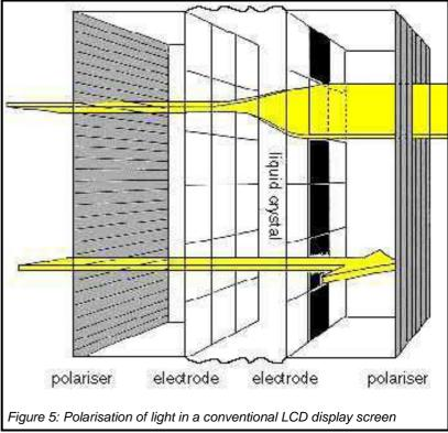
In a normal state, light polarised by the first filter passes through the liquid crystal, through the second filter and out of the cell. When a voltage is applied across the electrodes, the orientation of the liquid crystal molecules is altered and the rotation of light polarisation does not occur. The polarised light is now unable to pass through the cell as the second filter absorbs it. This part of the display now looks black.
